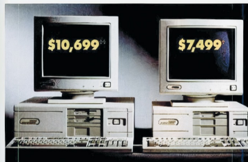
Compaq's 33 MHz and 25 MHz 386 computers. Systems include: VGA Color Monitor, 120 MB hard drive, 4 MB RAM.
